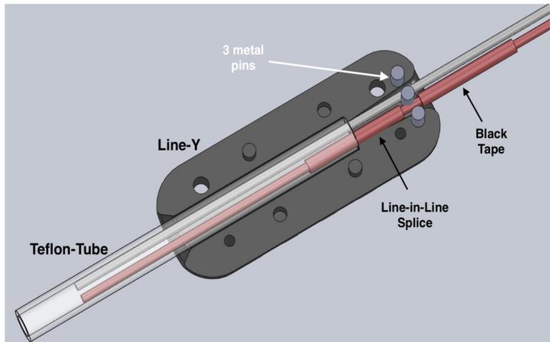
Please take care that the pins are exactly in the gap between the tape and the splice at the frontline with the black tape and line-in-line-splice.
